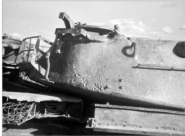
RPG "splatter" marks on the turret.
